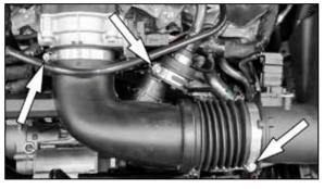
5. Loosen the three hose clamps that secure the intake tube and crank case vent tube then remove the tune from the vehicle
