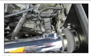
27. Reconnect the mass air sensor electrical connection.
