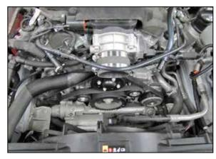
17. Install the provided coupler (084031) onto the throttle body and secure with the provided hose clamp.
