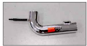
20. Install the EVAP hose assembly onto the K&N $^{\circ}$  intake tube as shown.
